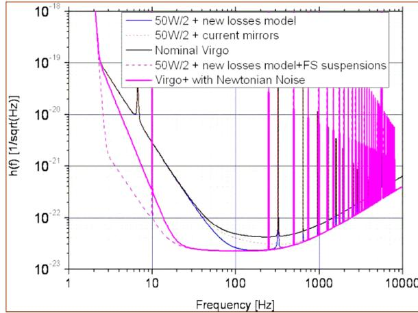
Figure6: Strain sensitivity comparison between the actual Virgo and the 50 W laser Virgo+
