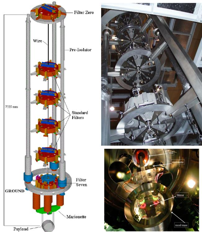
Figure3: The Virgo Superattenuator (SA)
