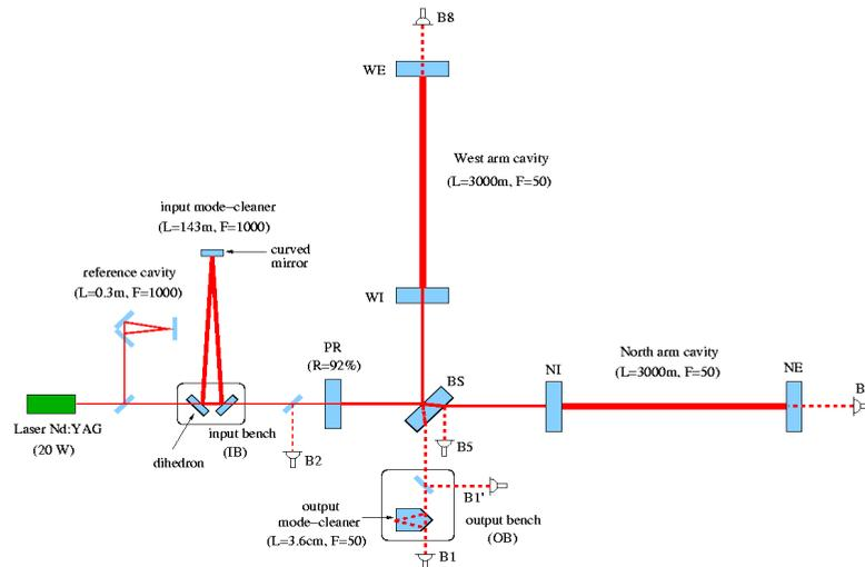
Figure 2: The Virgo interferometer optical layout
