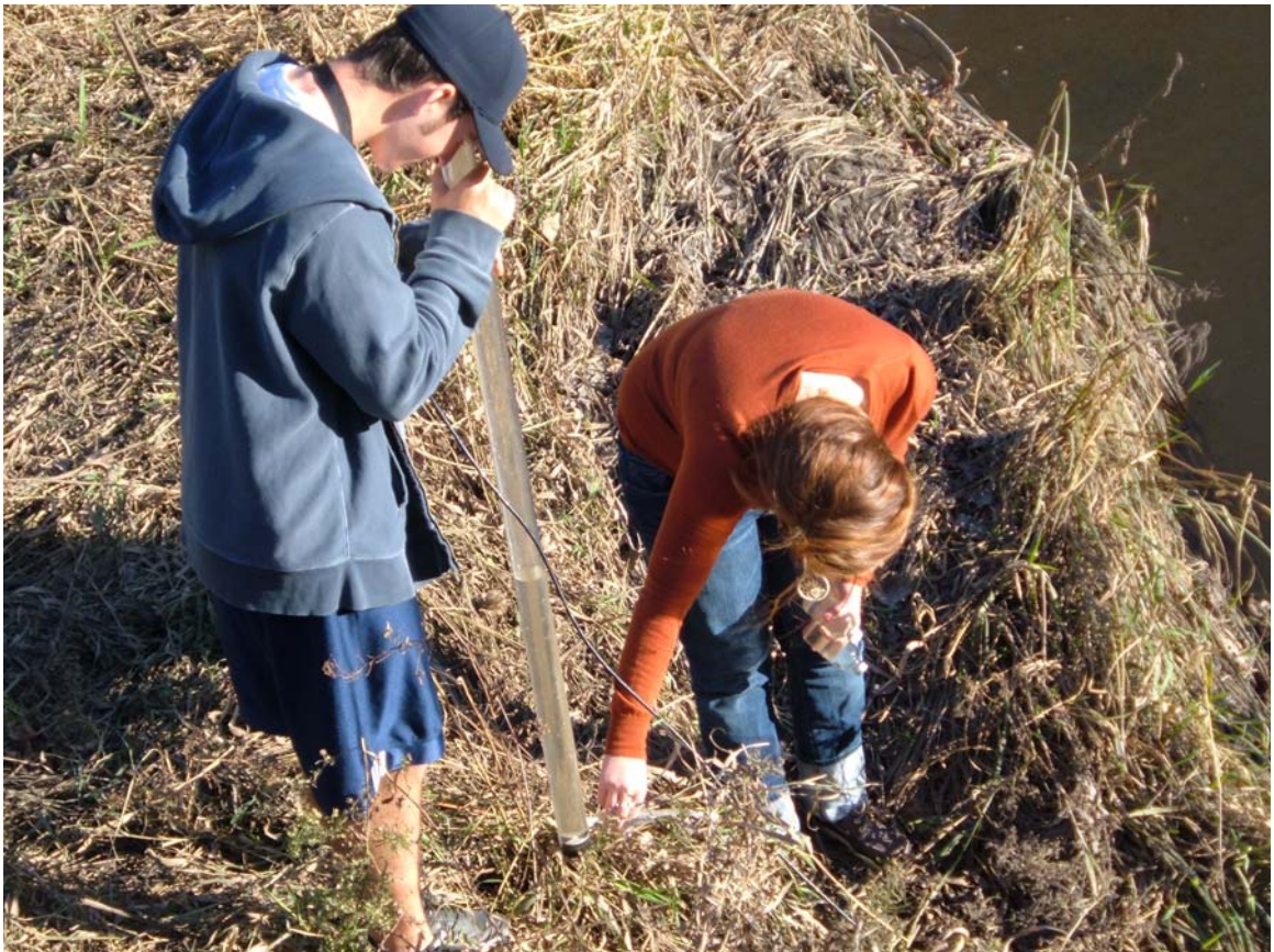
Image 2. Ted and Anna use the Secchi tube to measure turbidity; Anna is releasing the water while Ted looks to see if the black and white circle is visible.
