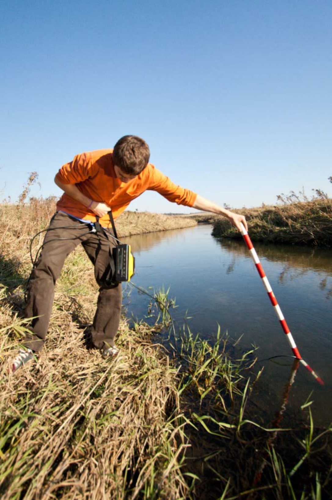
Appendix 7. Devin Holewinski using a flow meter to measure flow of Prairie Creek.
